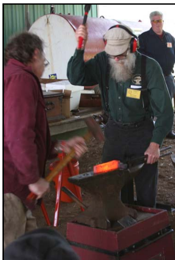
Tom Latané with Phil Heath striking on the forging die.
