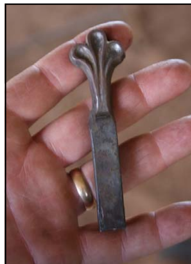
Master detail used to create forging die
