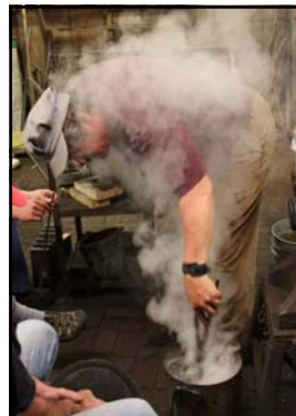
George demonstrating an oil quench!
