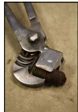
Universal Tongs made from channel lock pliers by Lee Thompson
