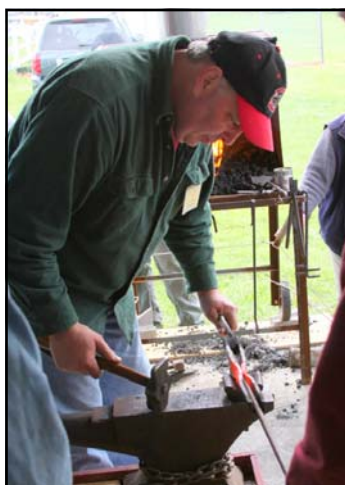
Richard Sullivan forge welding a gun barrel.
